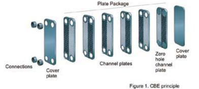
The fluids can pass through the heat exchanger in different ways. For parallel flow CBEs, there are two different flow configurations: cocurrent or counter-current.
