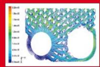
simulation is one of the most important stage in the development of new and existing CBE The ability to evaluate different plate patterns by simulating flow rate and directions offers great opportunities for improved functionality
